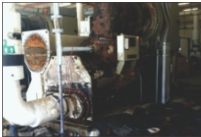
Original failed insulation removed
