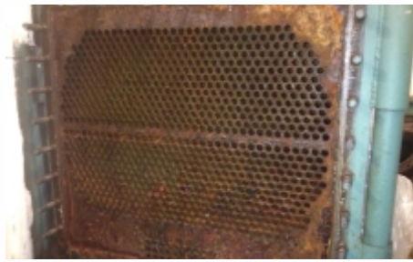
Tubesheet showing severe corrosion due to poor water treatment
